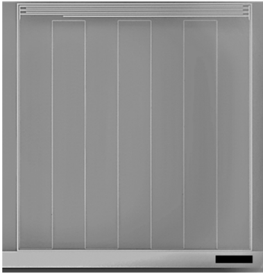
Fig. 2. SEM picture of a LEKID with size 3.2 \text{ mm} \times 3.2 \text{ mm} . Scale bar in black is 500 \mu\text{m} .
