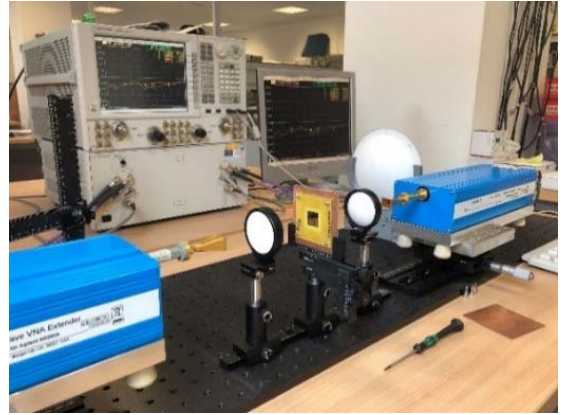
Fig. 6. Quasi-optical test-bench at W-band (75-110 GHz) for the LEKIDs characterization at ambient temperature.
