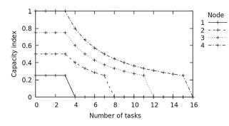
Fig. 1 Evolution of the index with increasing tasks on nodes with relative performances 0.25, 0.5, 0.75 and 1
