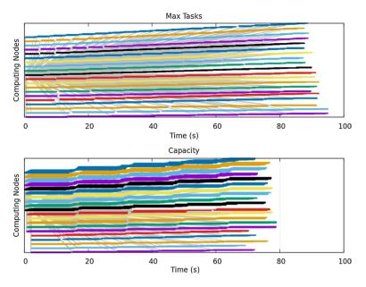
Fig. 4 Comparison of the task time distribution with Max-Tasks and capacity indices
