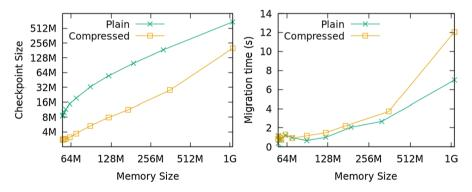
Fig. 5 Migration overhead with respect to the task memory footprint
