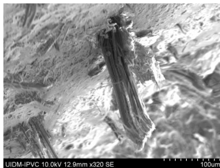
Fig. 6. Fiber-cement roofing sample of Afife, Viana do Castelo house with 320X magnification
