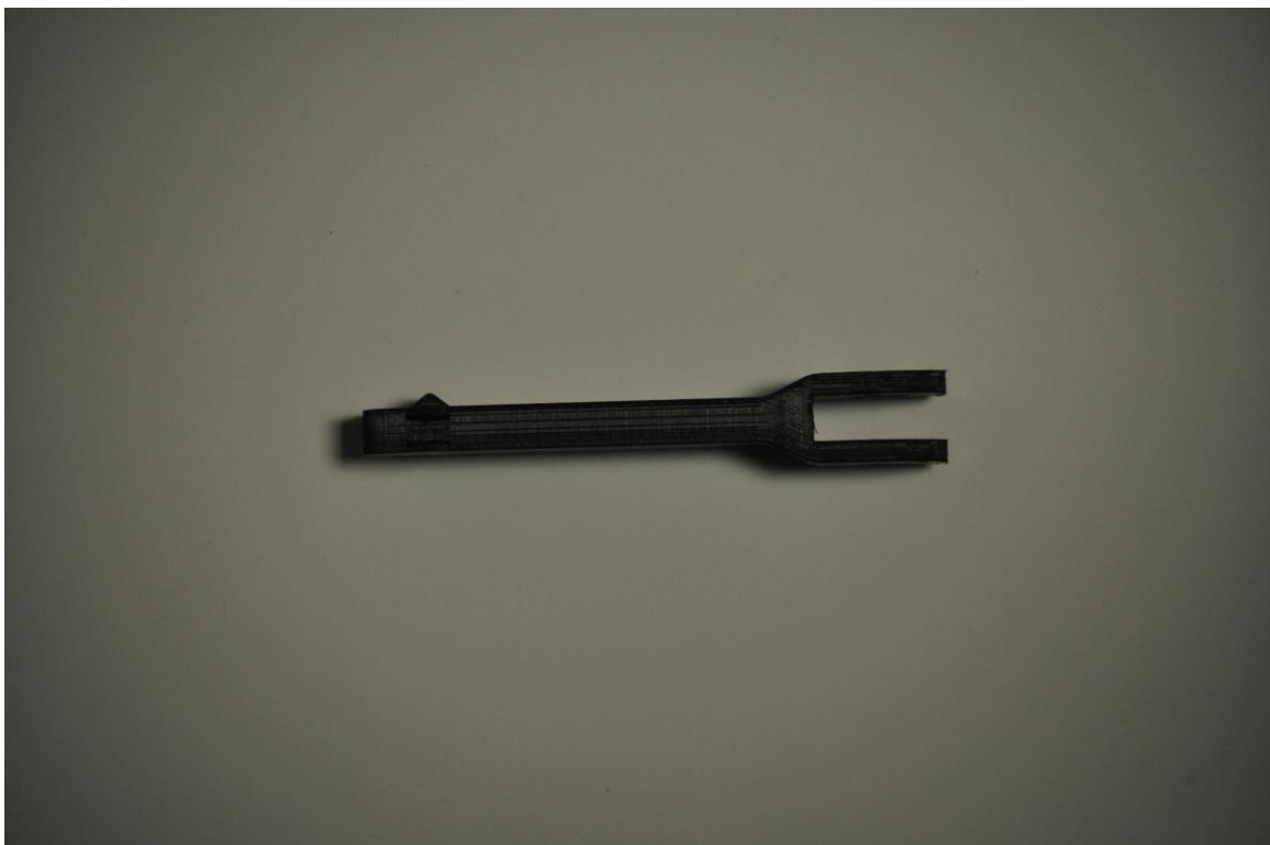
B.7 3D printed model of the lower leg of the device (at a distance of 120cm with a 80x lens).
