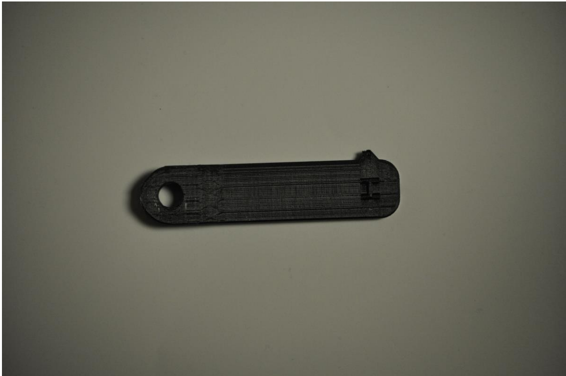
B.7 3D printed model of the lower leg of the device (at a distance of 120cm with a 80x lens).
