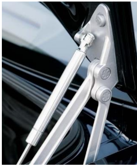
Figure 29- A trunk pneumatic mechanism, the inspiration for a smooth transition between stances [82].
