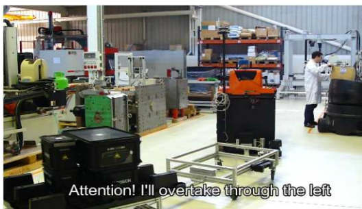
Fig. 1. Tugger and trailer assemblies operating a milk-run process on a dynamic factory floor shared with human operators.
