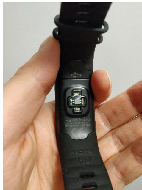
Figure 36. The PPG sensor of the Polar A370 heart rate monitor © Mikko Korkiakoski
