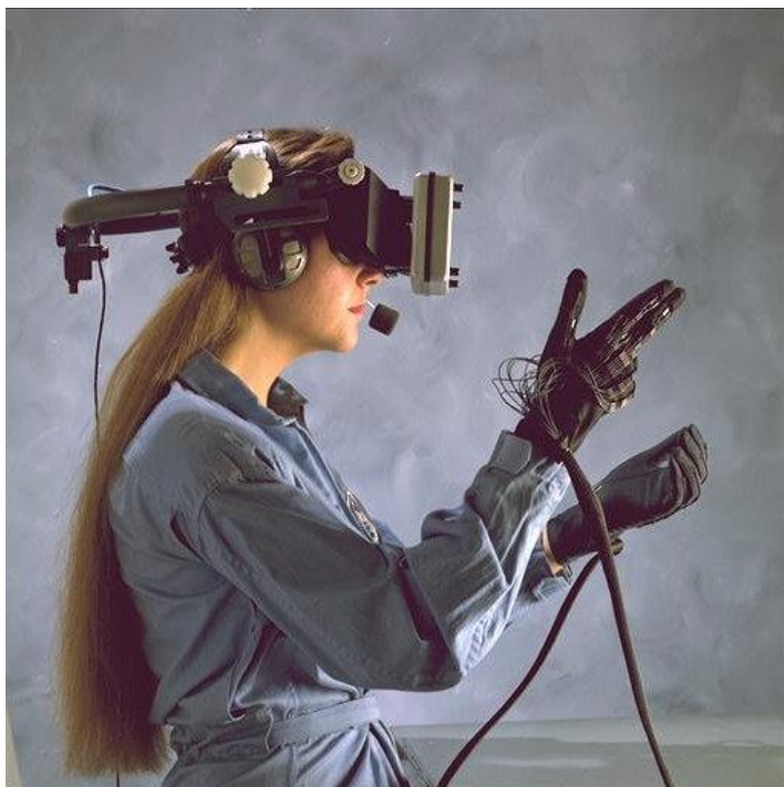
Figure 6. A woman wearing a head-mounted display incorporating Pop Optics goggles developed by NASA's Ames Research Center, and wired gloves © Public domain
