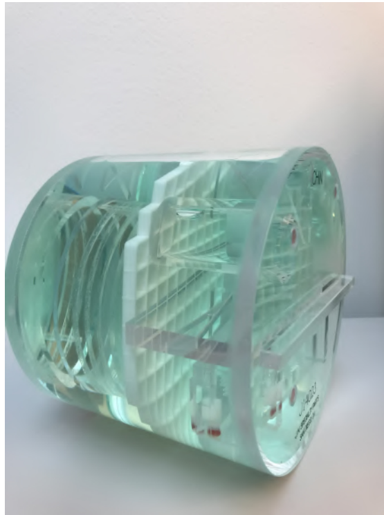
Figure 3.5: The ACR MRI phantom. The distortion grid is visible in the middle.
