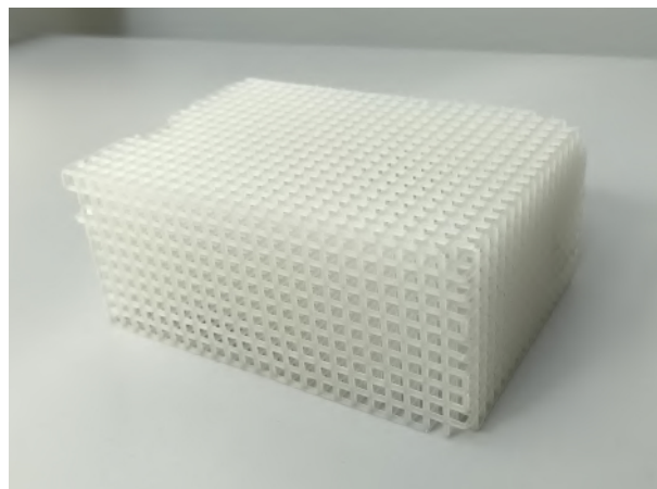
Figure 3.2: A sample piece of the 3D printed 5 mm grid.
