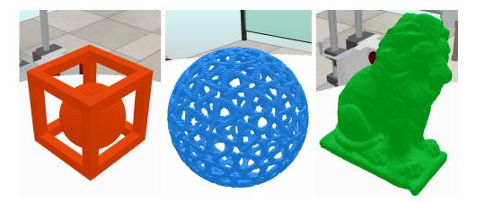
**Fig. 10** Examples of detailed printed 3D models using **FIBR3DEmul**. The cube printed with a filament width of 0.8 mm, the other two with filament width of 0.4 mm
