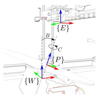
Fig. 9 Reference frames of the  $\{W\}$  world,  $\{E\}$  extruder, and  $\{P\}$  print table
