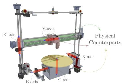
(c) C3DPrinter moving parts. Graphical and physical parts represented, as well as the position of each of the 5-axis.
