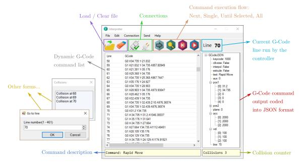
Fig. 1 Graphical user interface of the G-Code Interpreter application
