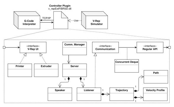
Fig. 7 UML diagram of the controller plugin
