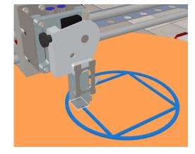
Fig. 5 Collision detected between the extruder and the printer table, which changed color to denote the occurrence
