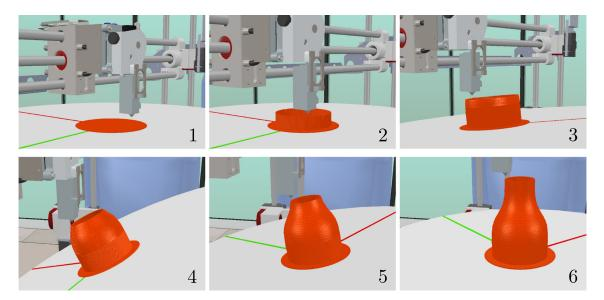
Fig. 11 Example of a 3D-printed model with 5 simultaneously actuated axes
