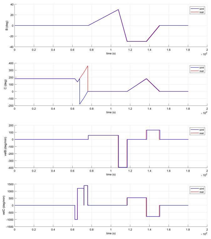
Fig. 13 Position and velocity plots of the print table axis of the virtual and the real "C3DPrinter"
