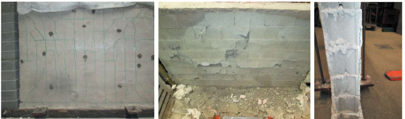
Figure 12 – Displacements evolution (Specimen 6): (a) Crack pattern on the unexposed face; (b) Spalling at the exposed face; (c) Vertical cracks at the middle of the wall
