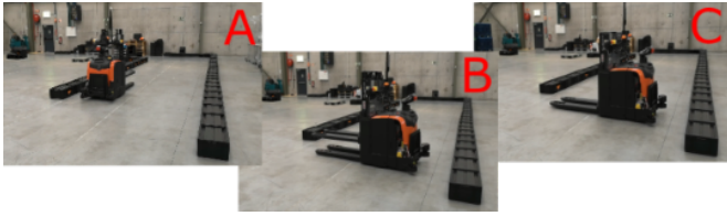
Fig. 12. Snapshots of experiment 2: Stacker operation cancelled due to absent pallet in loading zone. ( https://youtu.be/8clcmjCcc3E ).
