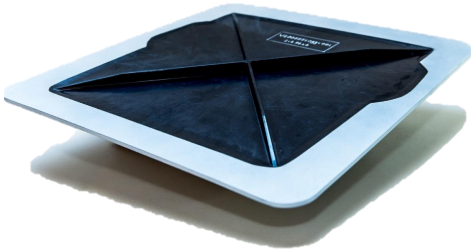
Figure 7. Developed demonstrator access panel for the rotorcraft
