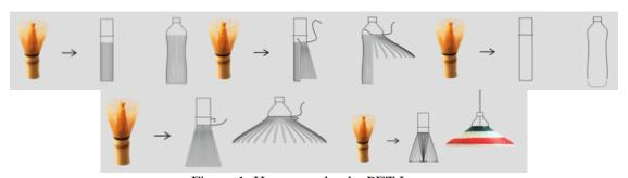
Figure 1: How to make the PET Lamp Source: <a href="http://catalandeocon.com/product/pet-lamp/">http://catalandeocon.com/product/pet-lamp/</a>
