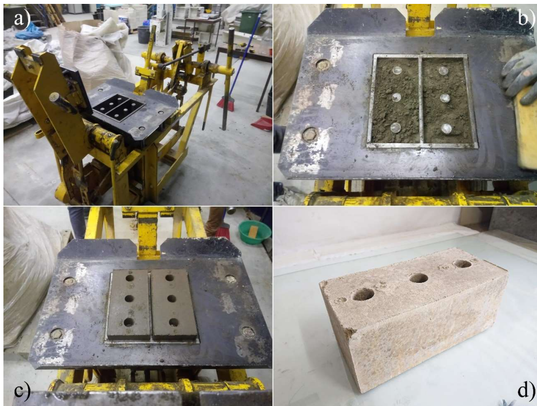
267 Figure 7. Main steps in the fabrication process of the CEBs, including, after mixture of the soil with the 268 alkaline cement, the filling of the moulds (a and b), the subsequent compression (c) and the curing and drying 269 of the resulting blocks (d)
