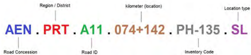
Fig. 2. Culvert code ID explanation – Relation between culvert geographic location and inventory code.
