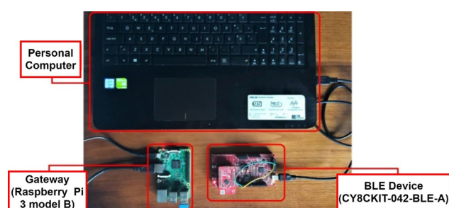
Figure 2. Main hardware components used in the development of the original smart home network.
