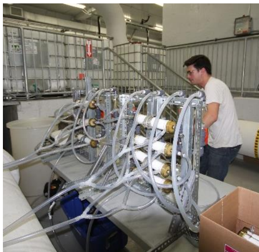
Figure 8-2: Installations with four Hemoflow-filters in parallel for the rapid concentration of microorganisms in large volumes of water
