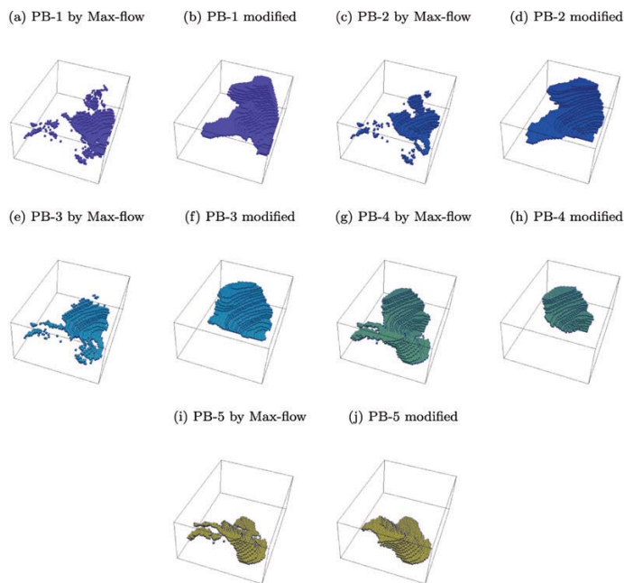
Figure 16—Case 2, comparison of modified pushbacks and original in 3D. The modified PBs become more cohesive, smoother, and regular. All isolated blocks or areas are filtered out
