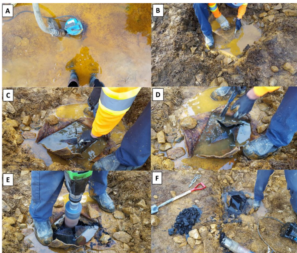
Figure G3 Different steps of LPR sampling at the inlet and the outlet of each treatment unit: A) Excess water removing, B) Gravel and straws layer removing, C) Geotextile cutting, D) Geomembrane cutting, E) LPR sample coring, F) LPR sampling
