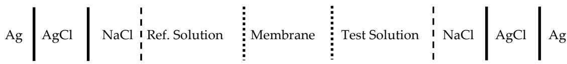
Scheme 1. Electrochemical cell based on ion-selective membrane electrodes for potentiometric measurements.
