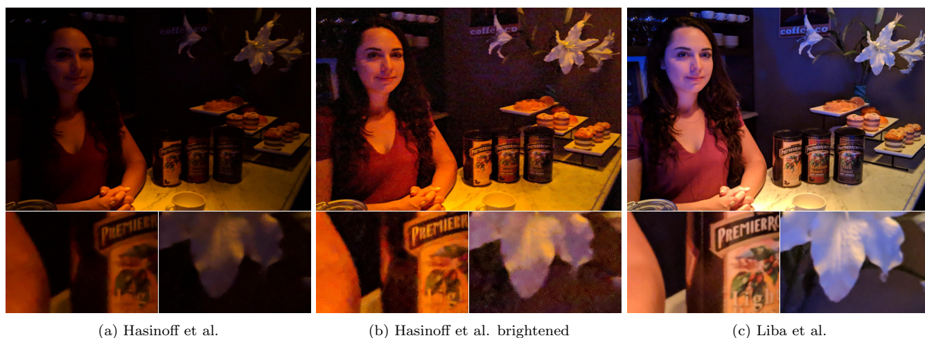
Figure 11: A comparison of images captured using the Hasinoff et al. pipeline (a and b) and the pipeline by Liba et al. showing the improvements in detail and noise from selecting a longer exposure time due to the low motion in the scene and taking more frames. It also shows the improvements in color reproduction from the improved white balance algorithm and tone mapping. [6]
