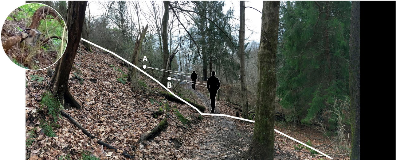
FIGURE 2 | Image depicting the field test location, looking toward the trail entrance, with the location of the PIC ( A ) and infrared trail sensor ( B ) noted. The PIC was 3 m from the trail edge and the sensor was 1 m from the trail edge. The inset photo is an image of the PIC mounted to sturdy grape vine at location ( A ). PIC, passive infrared camera. Bold line shows cross section of topography at infrared sensor location (foreground). Horizontal lines denote 0.6-m contours.
