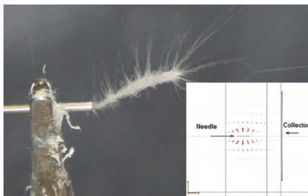
Figure 7. Visualization of the realtime fiber formation from a polymer droplet under electrostatic field and the verification of the electromagnetic field lines between the needle tip and collector surface separated by 15 cm at 15 kV potential. A close matching with experimental observation and field line simulation is presented here.
