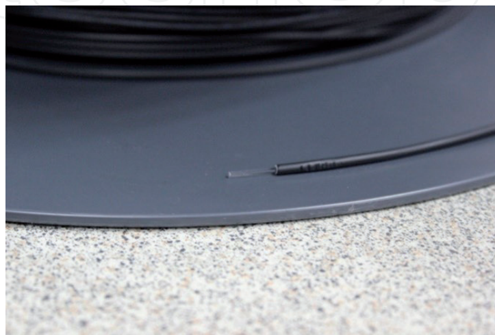
Figure 1. PMMA polymer optical fiber with diameter 1 mm.
