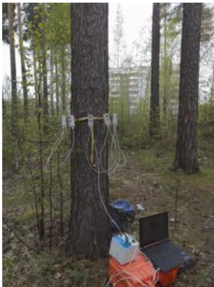
Figure 2. Arbotom® wood condition measurement.
