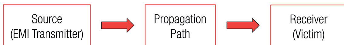
Figure 1. Main elements in electromagnetic interference phenomena.
