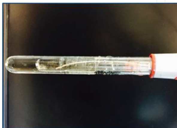
Figure 4. Jenway Ag/AgCl double junction reference electrode.
