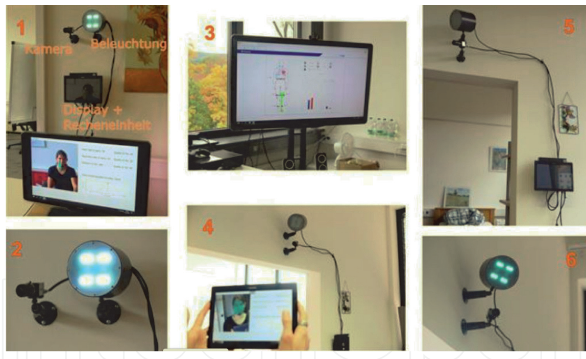
Figure 9. Camera-based vital sensors, 1 measurement unit, 2: Camera and lighting system 1, 3: Central display of real-time measurement 4: Measurement system 1 while application, 5: Measurement system 2 in while application, 6: Camera and lighting system 2.
