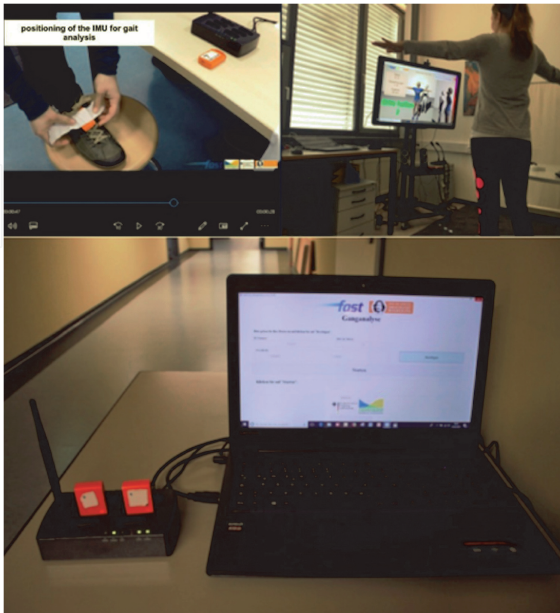
Figure 7. Setup of the gait measurements for e-rehabilitation of Otto von Guericke university; above left: IMU application at the feet; above right: Therapeutic movements with avatar; lower middle: Presentation of gait analysis measurement.
