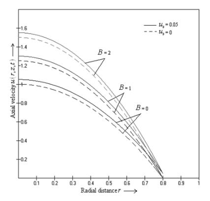
Figure 2. Variation of axial velocity with radial distance at z = 0 for different values of  $u_s$  and B with e = 1 and t = 1
