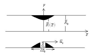
Figure 1. Schematic diagram of an artery with stenosis.
