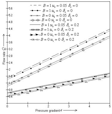
**Figure 4.** Variation of flow-rate with pressure gradient for different values of  $B, u_s$  and  $\delta_s$  with t = 1
