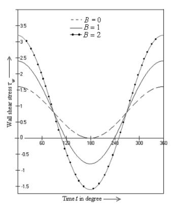
Figure 5. Variation of wall shear stress with time for different values of B with e = 1, and  $\delta_s = 0.2$
