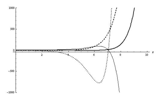
Figure 6. Perturbation quantities  $h_1$  (thin solid line),  $v_1$  (dashed line),  $\sigma_1$  (thick solid line) and  $E_1$  (dotted line) versus the axial variable z for  $\Omega = 4$ ,  $\sigma_0 = 0.1$ , t = 1, k = 0.2, s = 1.3921 and  $\omega = 0.1603$ .
