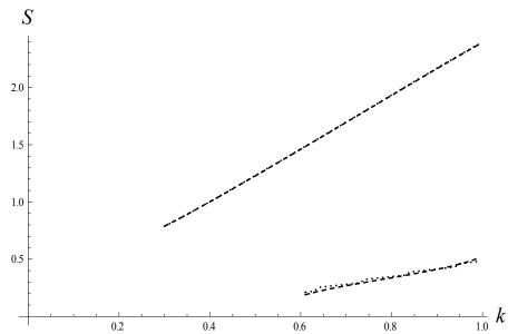
Figure 1. A comparison of the numerically computed results for the growth rate S versus the wave number k for very large conductivity  $K^*=10^5$  (dotted lines) and the asymptotic results due to Riahi (2009) for  $K^*=\infty$  (dashed lines). The values of the other parameters in this comparison are  $\nu = 0.333$ ,  $\beta = 77.0$  and  $\sigma_0 = 0.1$ .
