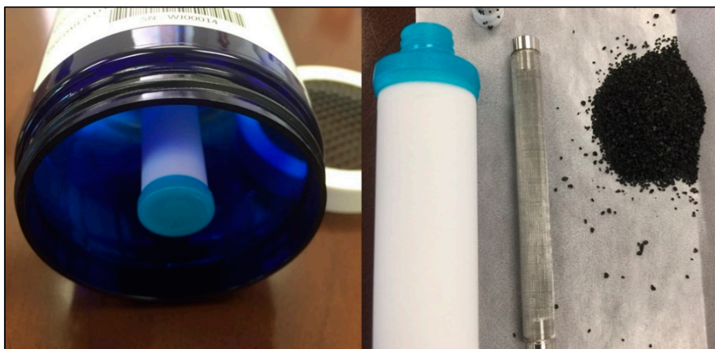
Figure 2. Photos showing the Hg passive air sampler (MerPAS) with a White Radiello diffusive body inside a protective shield and the mesh cover in the background ( left ), as well as a close up of the diffusive body, stainless steel mesh screen, and sulfur-impregnated activated carbon sorbent ( right ).
