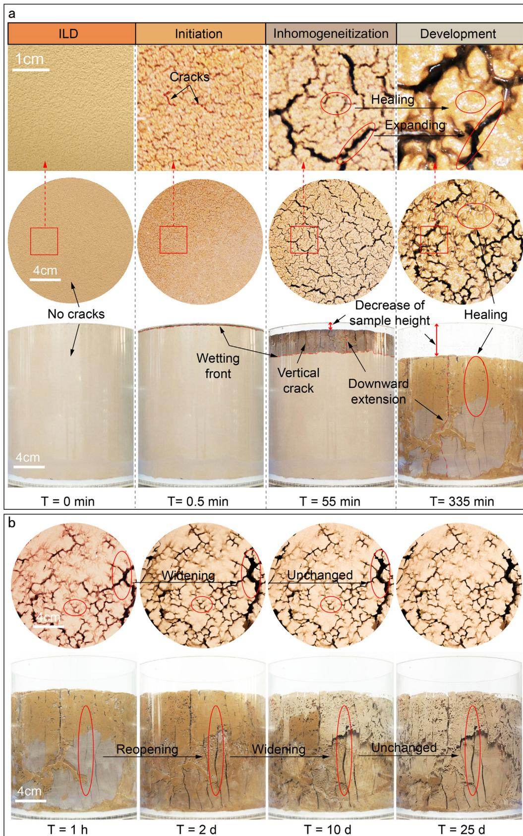
**Fig. 3.** Structural evolution of ILD during WD cycle as viewed from the top and sides of the sample. a, Main stages of ILD's structural evolution during wetting (crack initiation, inhomogeneitization, and development). b, Structural evolution during drying.
