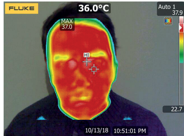
Figure 2 Combined passenger image in the visible and infrared wavelengths at a distance of 0.5 meters
