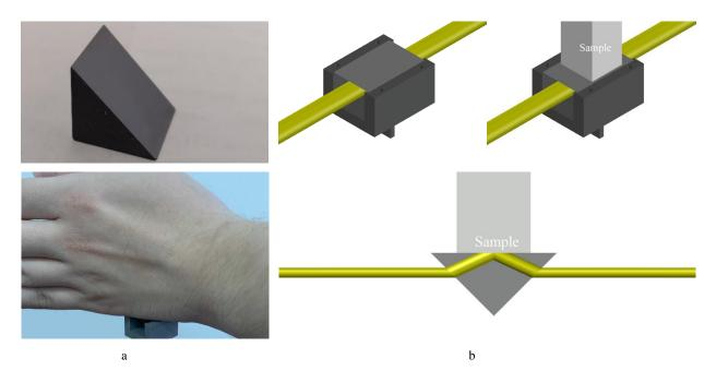
Figure 2 - Prism ATR (a), the reflection scheme (b)
