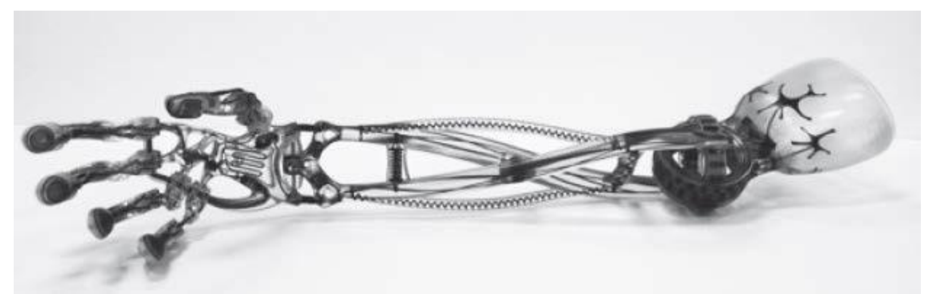
Figure 4. Multi-functional multi-material prosthetic arm
