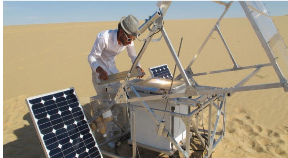
Solar-powered AM creating crude glass out of sand in the Sahara desert
