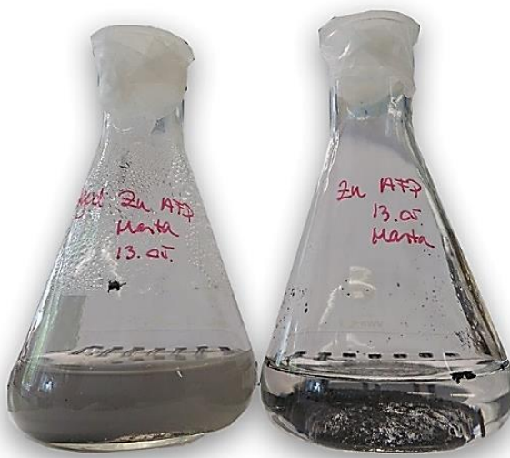
Figure 7. 72-hour leachate of weathered paint microparticles (left-hand side) and the leachate of non-weathered paint microparticles of the same material (right-hand side).
