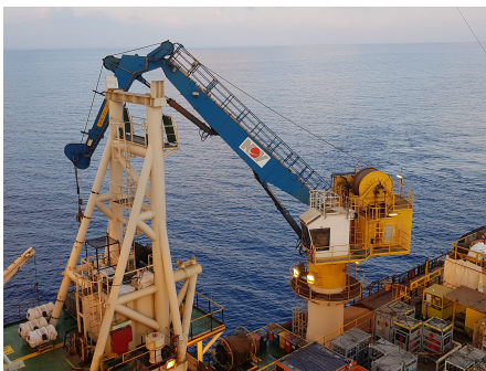
Figure 1.1: A 25 ton knuckle-boom crane. ©NOV, Geir-Arne Moslåttn 2018.
