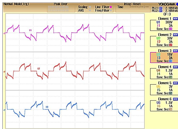
Figure 20. Voltage source inverter-fed BLDC motor output current waveform.
