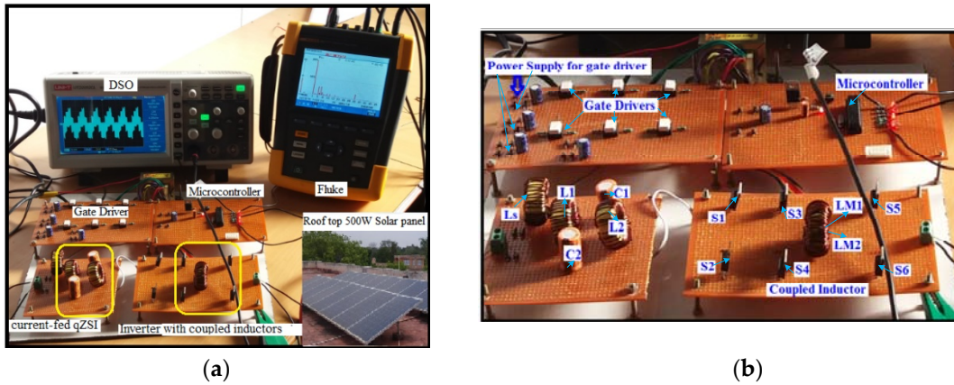
Figure 40. Experimental setup; (a) overall laboratory-scale 500 W PV powered modified Q-impedance fed coupled inductor MLI, (b) modified Q-impedance fed coupled inductor MLI.
