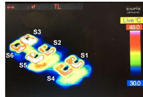
Fig. 19. Thermal image of the PUC converter by applying the traditional modulation method.
