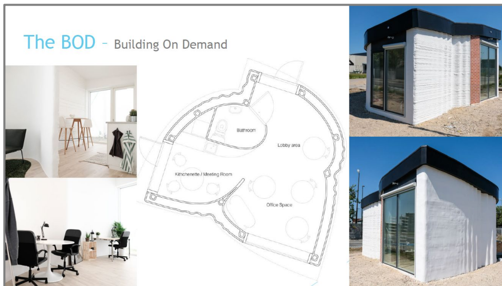
Figure 50. Presentation 5 by Ellinghausen on the first European 3D printed building BOD produced by COBOD in 2017.
