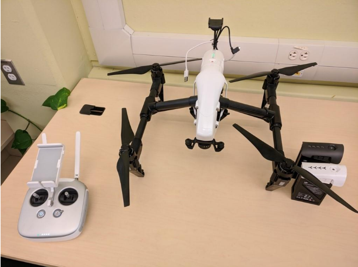
Figure 2: DJI Inspire 1 multi-rotor quadcopter with the DJI Inspire controller and batteries.
