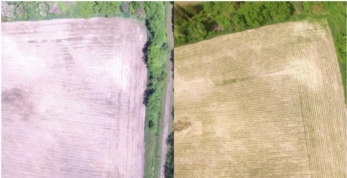
Figure 17: (Left) Image acquired by the RPAS during high brightness conditions, (Right) Image acquired by the RPAS during normal brightness conditions
