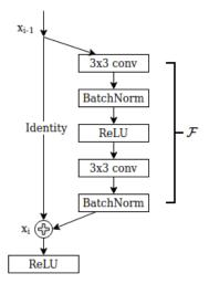
Figure 2. Residual Block from ResNet [25]
