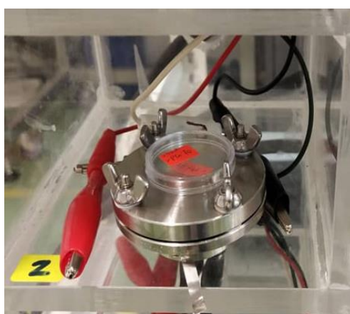
Fig. 2. PANI/GO nanocomposite electrodes were assembled in a battery jig for electrochemical testing
