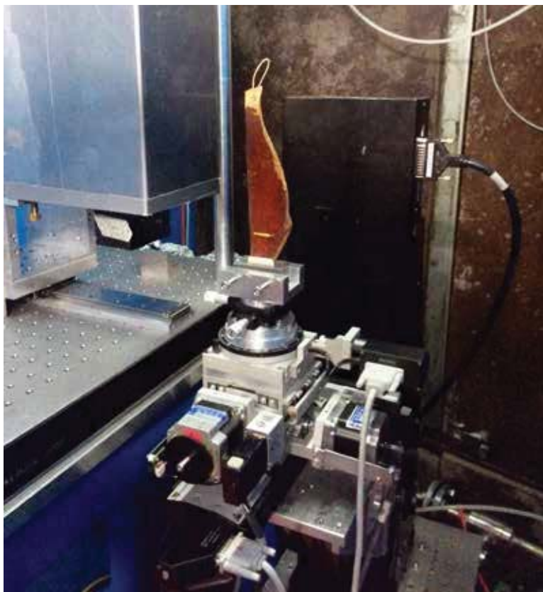
Figure 1: Tomographic setup of the high-resolution SR-micro-CT in phase-contrast mode at the SYRMEP beamline at Elettra.
