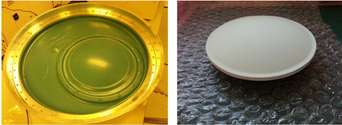
Figure 7. Left – image of coating rig. Right – example of a coated lens
