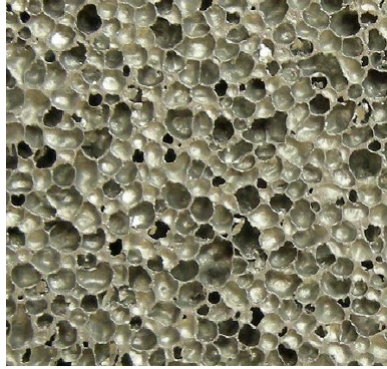
Fig. 1.1 Section of closed-cell foam
