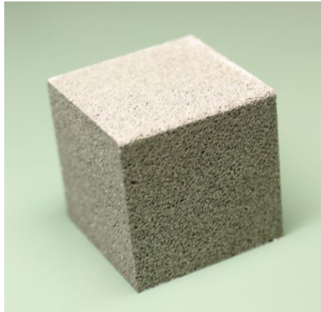
Fig. 1.9 Photograph of a titanium foam specimen fabricated by Powder metallurgy of side 22 mm.
