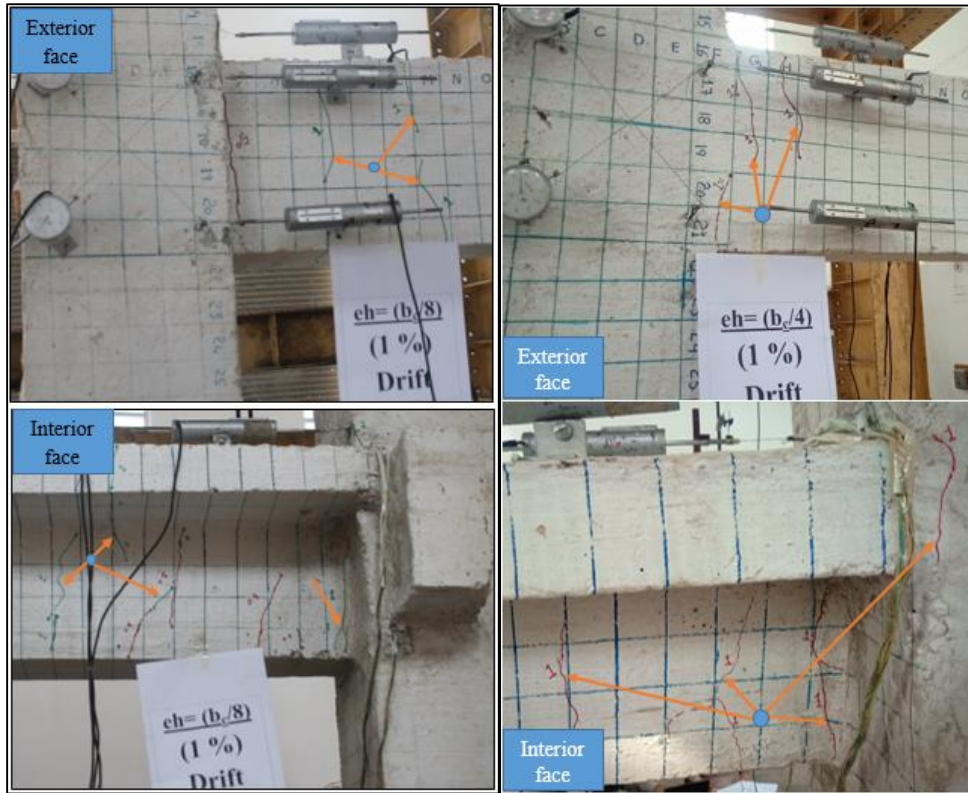
Figure 10. Crack pattern of specimen 1 (bc/8) and specimen 2 (bc/4) at 1% drift
