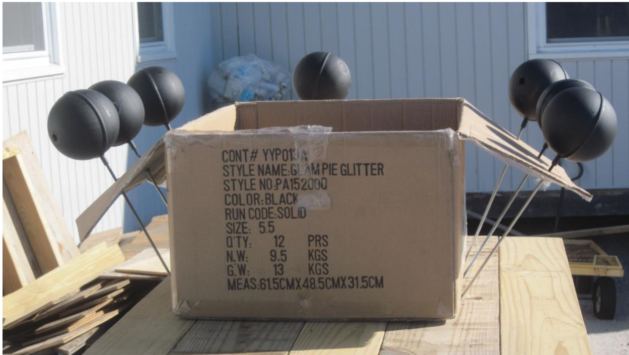
Figure 3. Vernon globe thermometers that were mounted on each station. Each copper sphere was painted matte black and contained an Onset 12-bit Smart Sensor thermistor.
