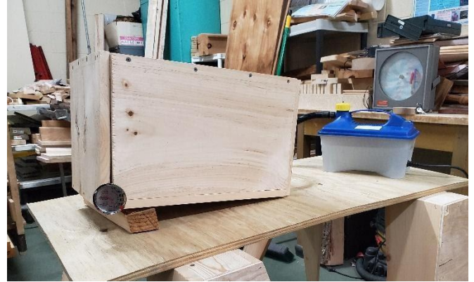
Figure 16: Pine Box and Rockler Steam Generator set up
