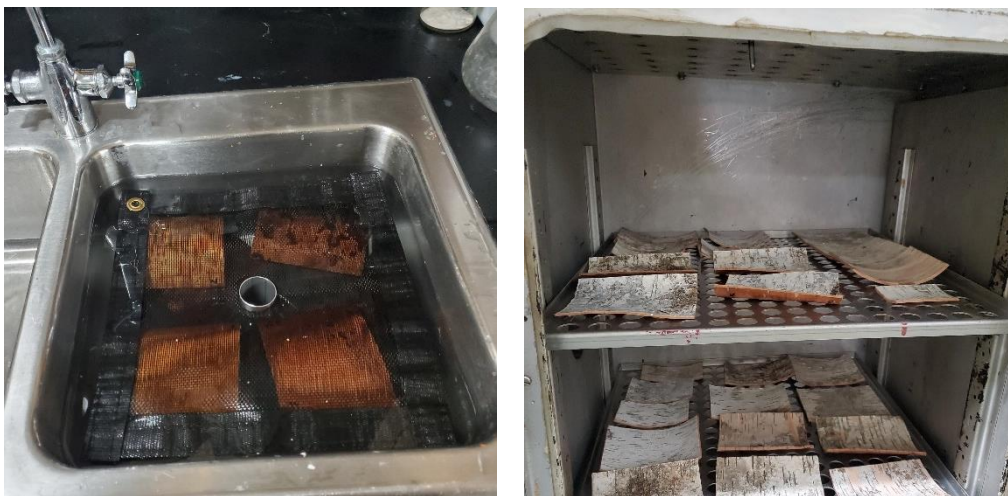
Figure 21: Samples in both conditioning environments, submerge and climate control chamber
