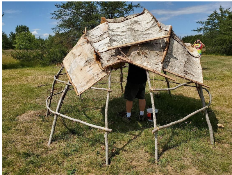
Figure 12: Wigwam structure for site exposure test
