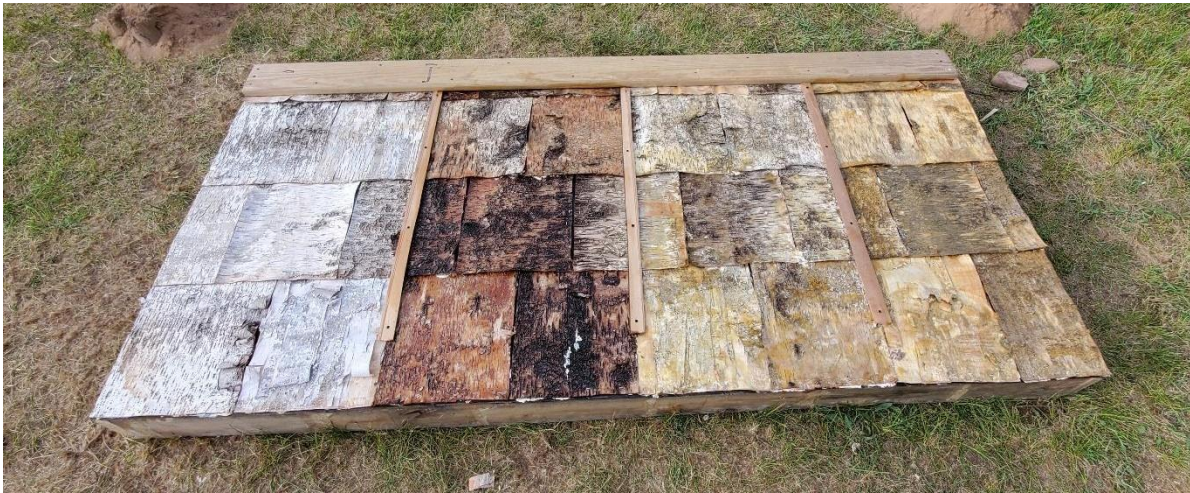
Figure 14: Sloped roof with finishes. Left to Right: Control, Sunflower Oil, Pine Resin, Thompson's Water Seal
