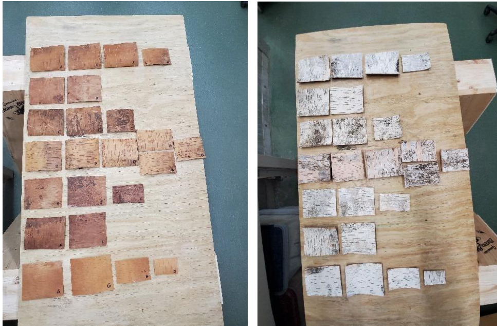
Figure 20: Front and back of samples for C120 and D3462 tests
