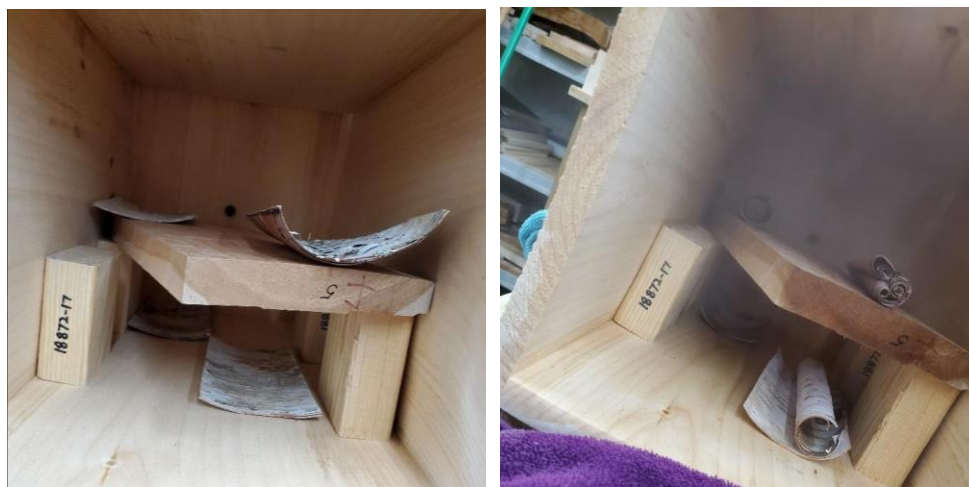
Figure 17: Comparison of birch bark samples at start and 30-minute check during steam test
