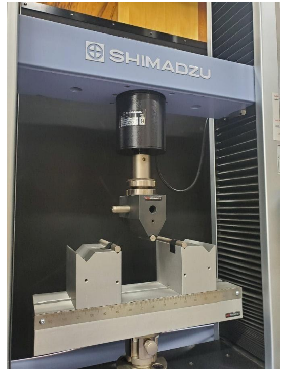
Figure 22: Shimadzu Testing Machine, model AG-X, prepped for three-point bending test
