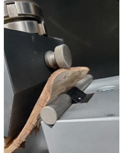
Figure 34: Example of Sample running into knob during Shimadzu testing
